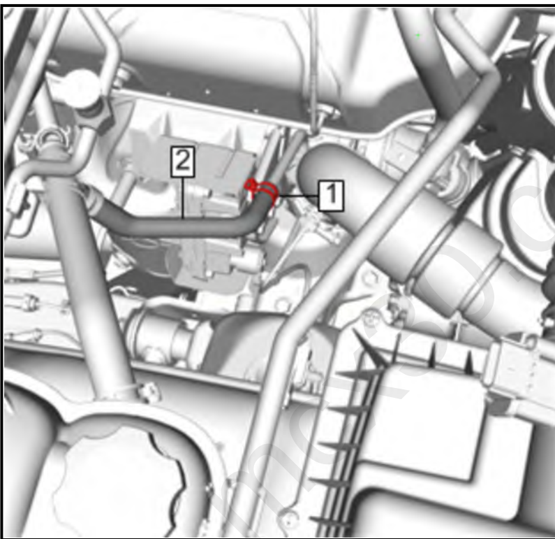
3. Radiator Surge Tank Outlet Hose (2) @ Turbocharger Coolant Return Pipe - Disconnect
